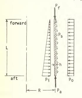
P<sub>f</sub> is the force per unit circumference along the forward edge and is associated with the acceleration of the forward structure.
